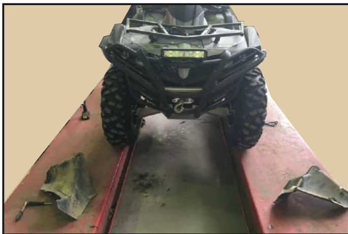
Remove the back cover of the headlights
