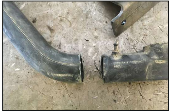
Saw part of the rear air intake tube as the sample
