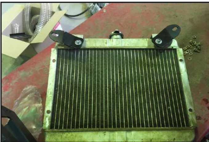
Install the brackets on the radiator
