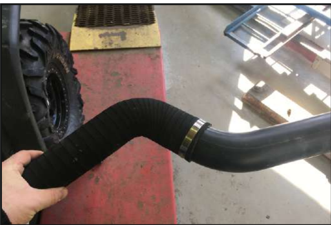
Install the adapter on the air intake tube part
