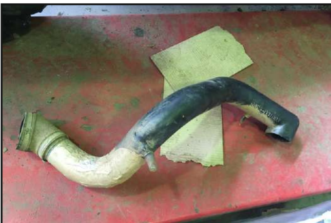
Take rear variator air intake tube
