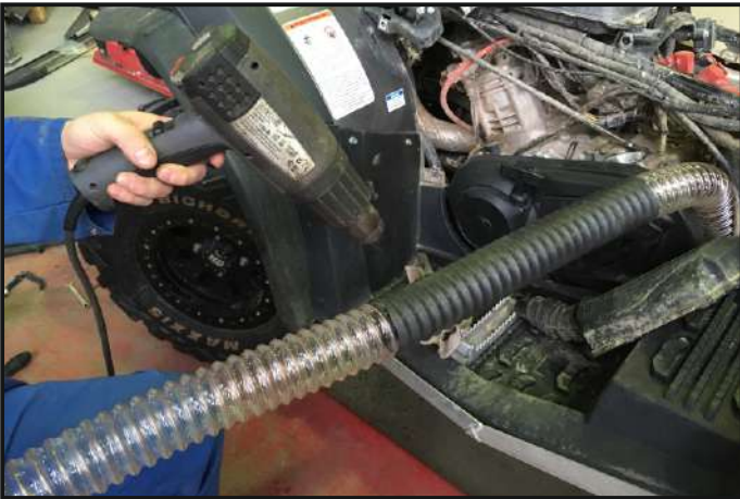
Install heat shrink tube along the engine
