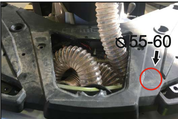
Drill a hole in the front rack panel lid d55-60mm
