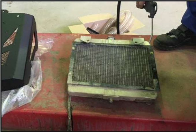
Clean the radiator
