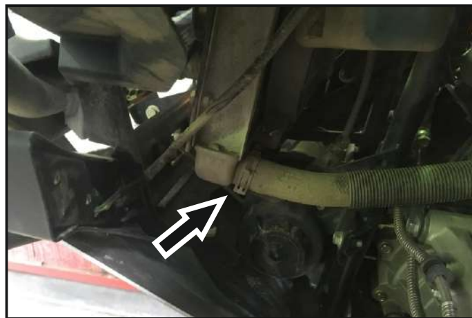
Remove the hose. Drain the antifreeze
