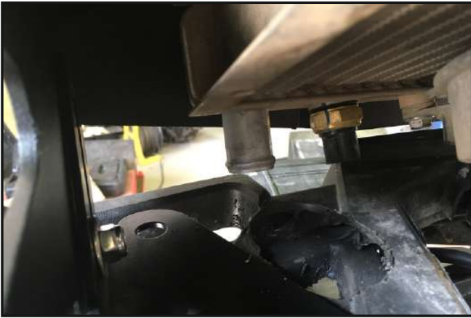
Install the straight hose from relocation kit MP0388
