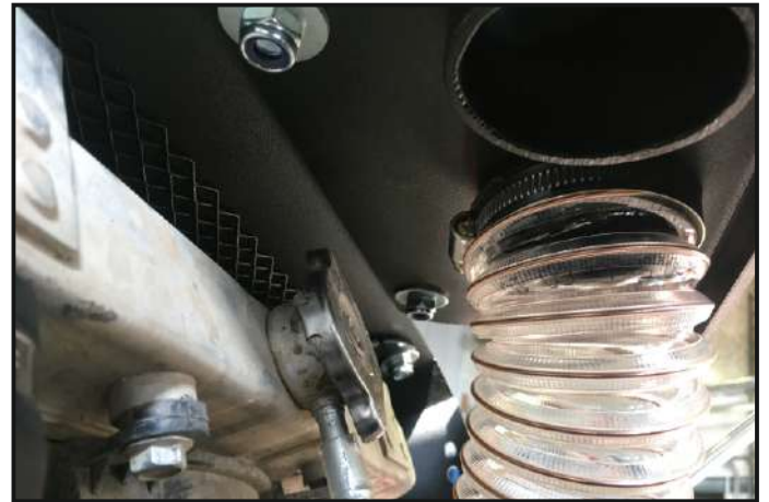
Install the corrugation on the snorkel head
