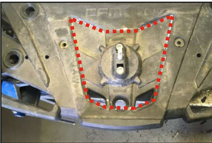
Cut out part of the front rack panel
