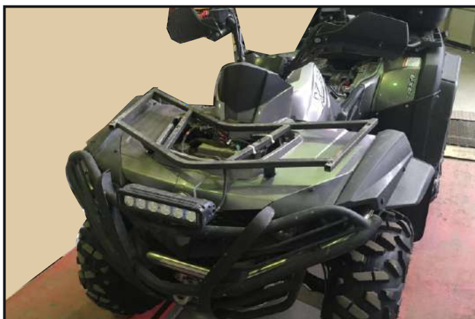
Remove the front rack panel
