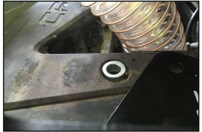
Install the bushing
