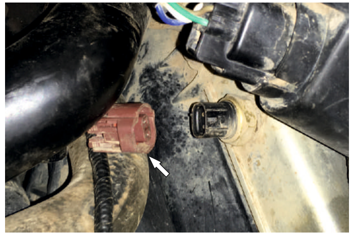
Unplug the temperature sensor connector and disconnect the connector of the radiator fan
