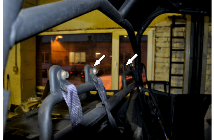
Unscrew the upper safety belts bolts
