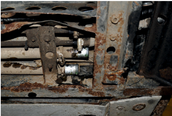
Remove radiator hoses under the UTV
