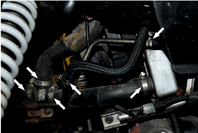
Remove hose filler neck, right hoses Remove oil radiator hoses
