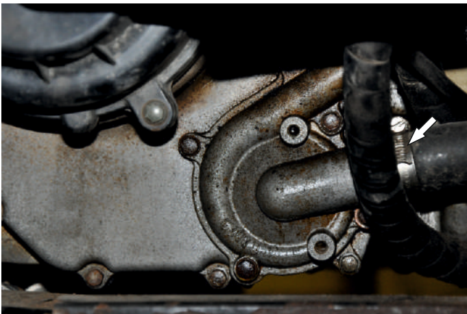
Unscrew and remove lower hose on engine
