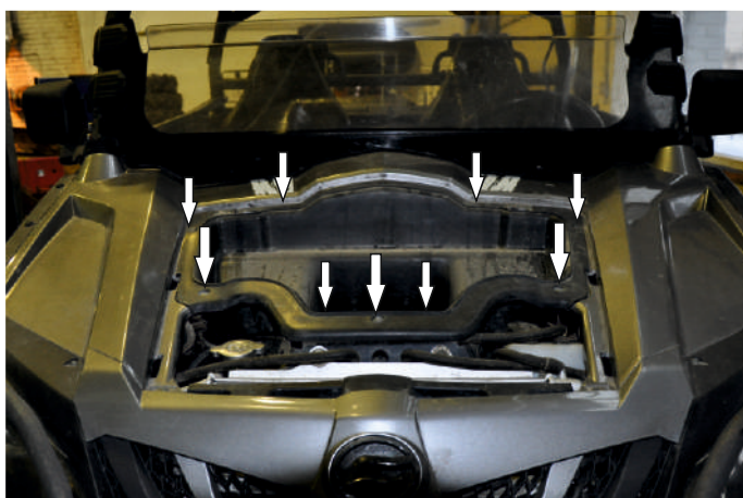
Unscrew and remove the front box
