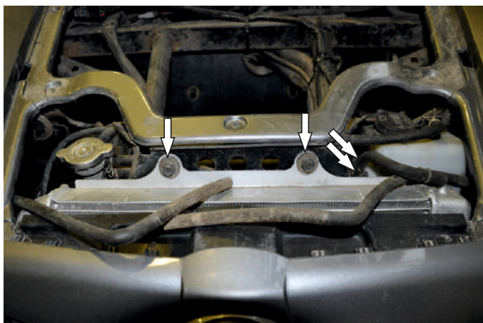
Unscrew the radiator mount and expansion tank
