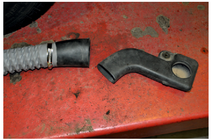
Saw the air intake tube as the sample
