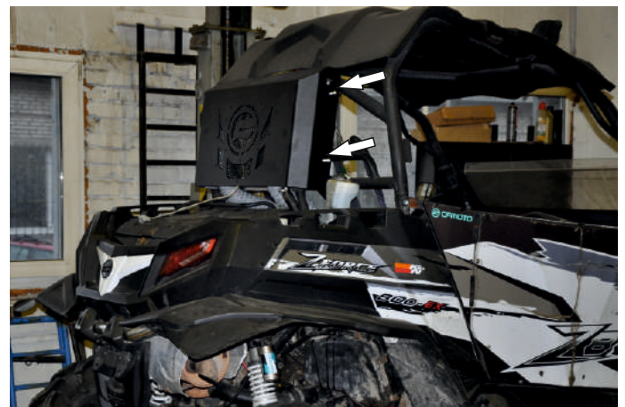
Tighten the relocation box cover
