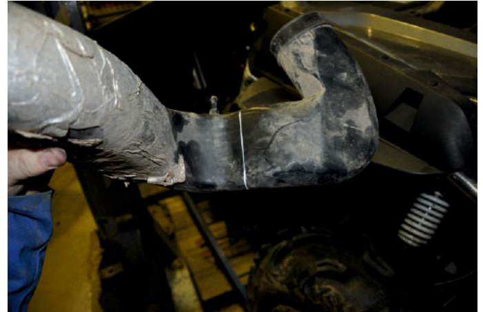
Saw the intake variator tube as the sample
