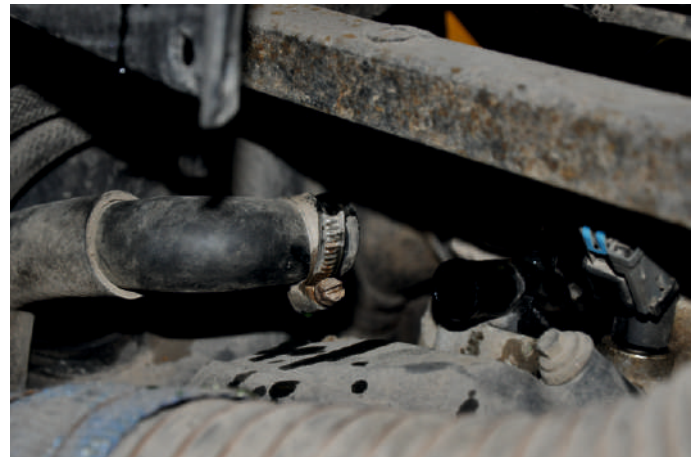
Unscrew and remove upper hose on engine
