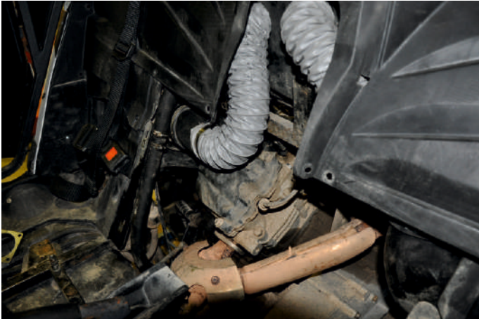
Connect the corrugation with a piece of air intake tube
