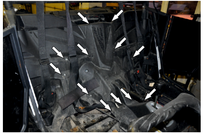
Remove the central interior panel
