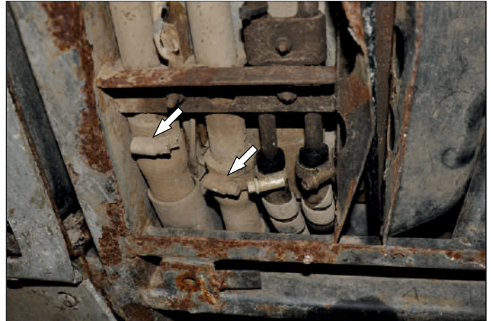
Unscrew radiator hoses under the UTV
