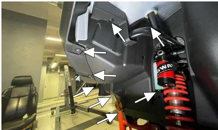
Unscrew the bolts and remove the plastic clips securing the left headlight trim in the front fender. (the right side is similar).
