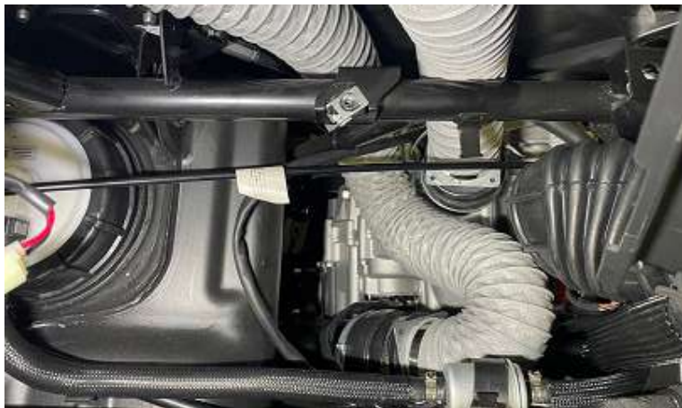
Lay the air ducts as shown in the picture.
