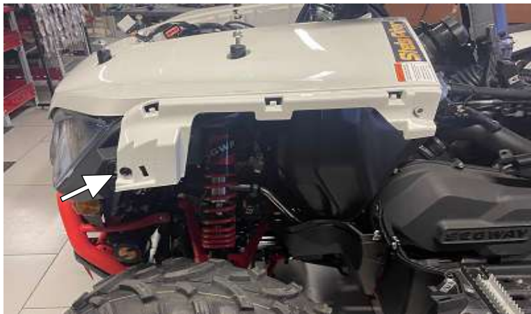
Unscrew the bolts of the front plastic. (the right side is similar).
