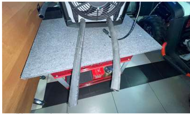
Install hoses to the radiator.
