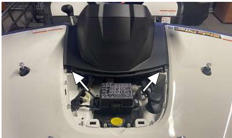
Unscrew the bolts on the dashboard cover.
