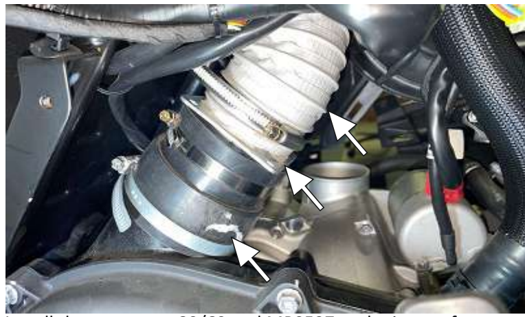
Install the connector 80/60 and MP0527 at the input of the variator housing. Install a flexible duct.
