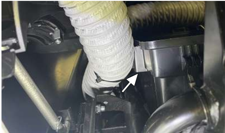
Tighten the duct with a plastic clamp. The rocker link should not touch the air duct.
