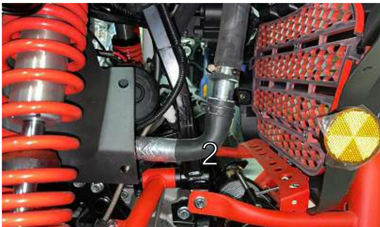
Connect the hoses to the cooling system.
