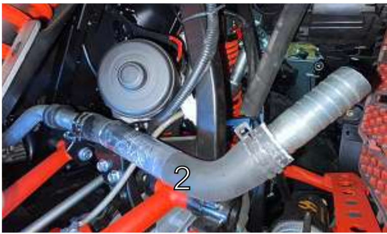
Set the element "2" to the right side. Install the hose connector.
