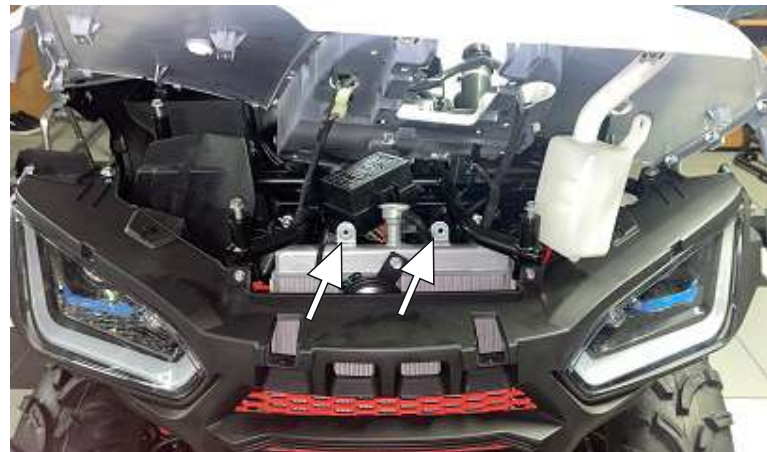
Unscrew the radiator mounting bolts.
