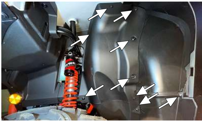
Unscrew the bolts and pull out the plastic clips of the inner panel of the left arch (the right side is similar).
