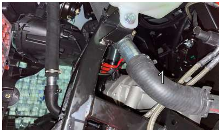
Connect the hoses to the cooling system.
