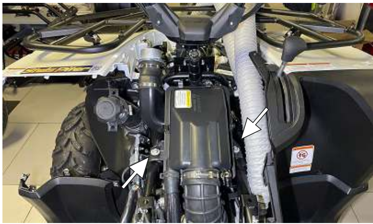
Screw on the air filter housing and install the cover.
