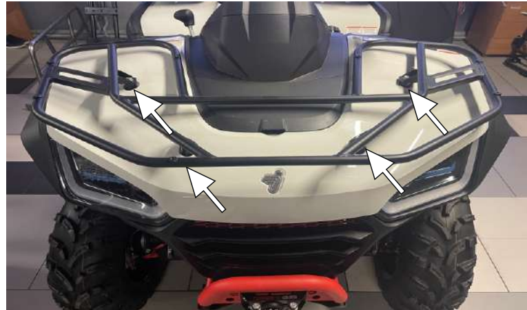
Remove the plastic cover of the front rack. Remove the front rack.
