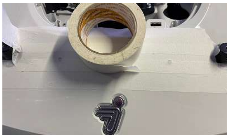
Glue the masking tape to the front plastic. As shown in the picture.
