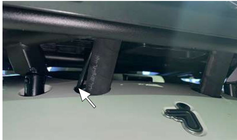
When installing, pass the hoses through the holes in the panel. Connect the cooler wire through the holes in the panels.
