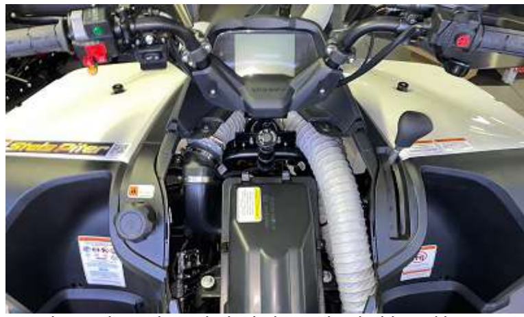
Pass the air ducts through the holes in the dashboard lining. The air ducts should not be clamped.
