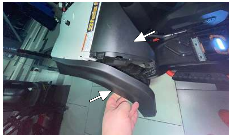
Remove the front fender trim. (the right side is similar). Remove the front left front fender panel.
