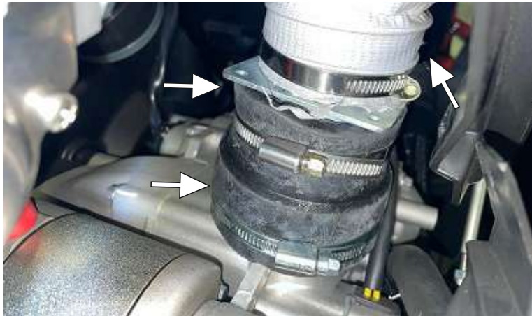
Install the connector 80/60 and MP0527 at the output of the variator housing. Install a flexible duct.
