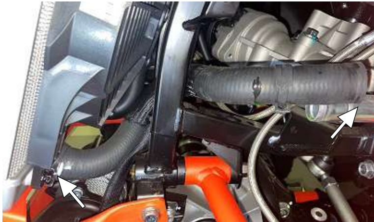
Remove the standard radiator pipes. Disconnect the fan connector.
