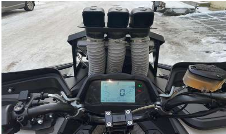
Install a panel with snorkel caps. Connect air ducts to them.
