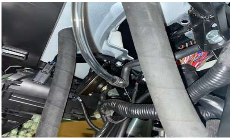
Lay the overflow tube as in the picture.
