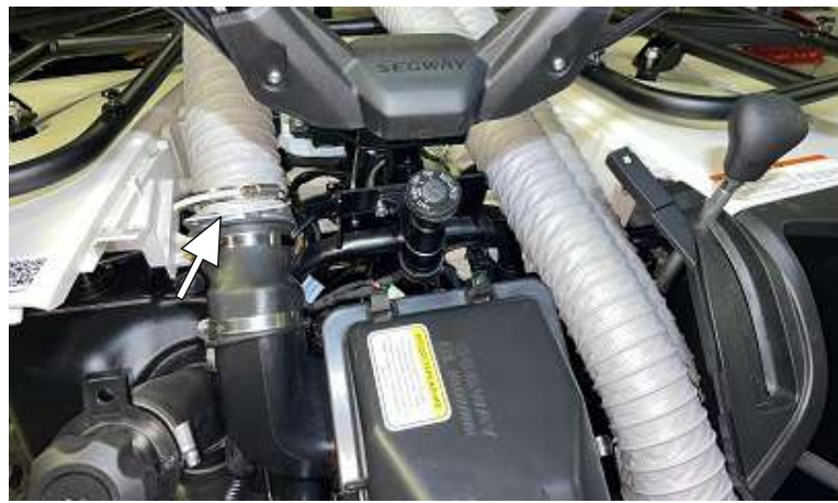
Install the air duct
