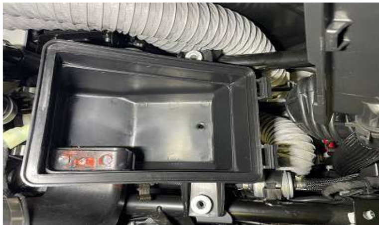
Install the air filter housing. Connector with the throttle.
