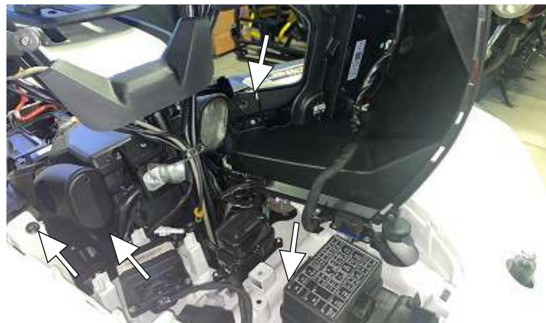
Unscrew the bolts of the front plastic. Remove the pipe of the CVT housing.
