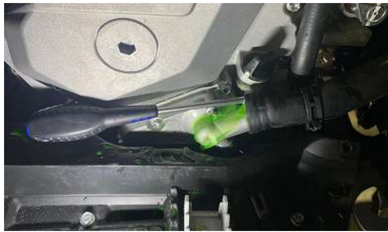
Put a tank under the ATV for antifreeze. Remove the nozzle and drain the antifreeze.
