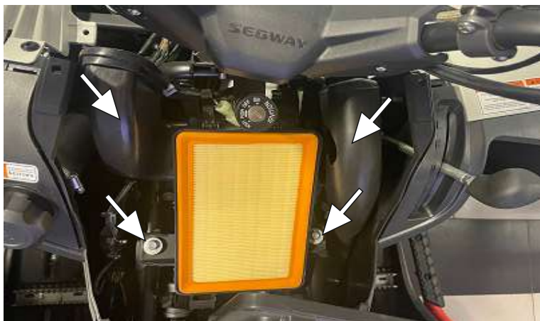
Remove the air filter lining and air filter cover. Unscrew the housing and throttle connection, remove the pipes of regular snorkels.
