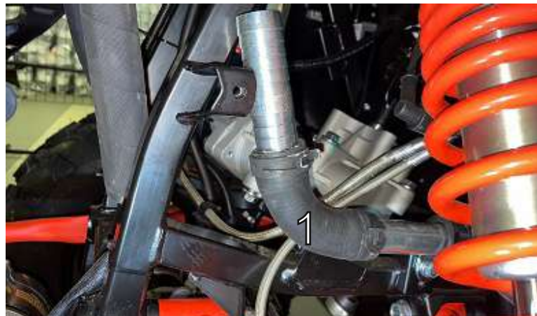
Set the element "1" to the left side. Install the hose connector.
