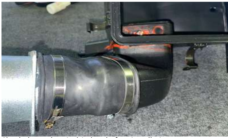
Check the sealant is dried up before installation.
