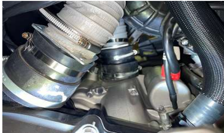
Install the connector 80/60 and MP0527 at the input of the variator housing. Install a flexible duct.
