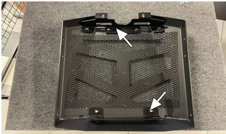
Install the upper and lower mounts on the radiator housing.
