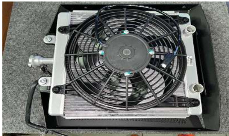
Install the radiator with the fan and fix it.
