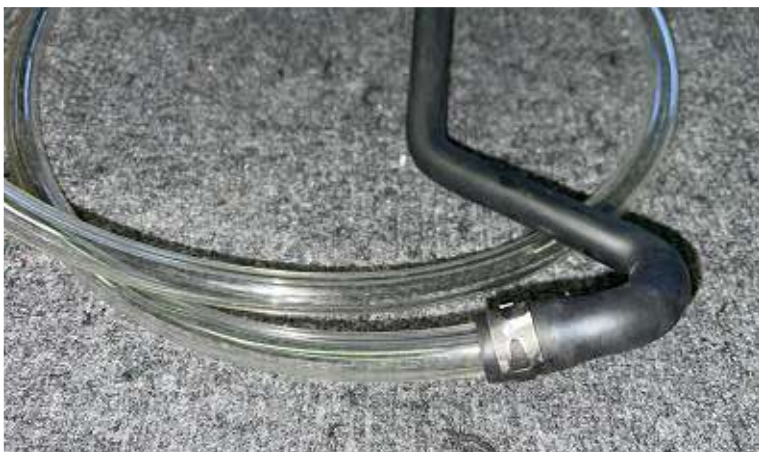
Extend the overflow hose with a piece of polyamide tube.
