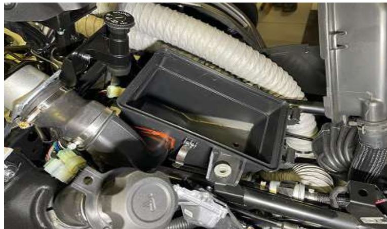
The duct MUST NOT BE clamped
