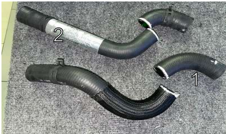
Cut the standard radiator pipes as shown in the picture.
