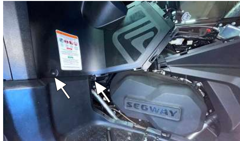
Unscrew the bolts securing the left front fender. (the right side is similar).
