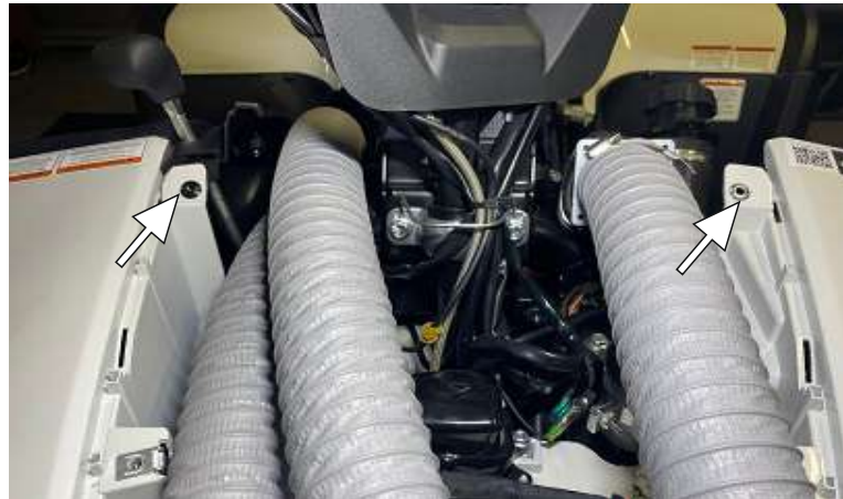
Install the air filter lining. Lay the air ducts as shown in the picture
