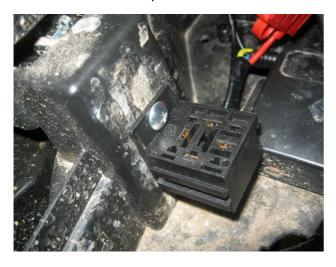
12) Eject the central panel for Auxiliary equipment and disconnect the connector;
