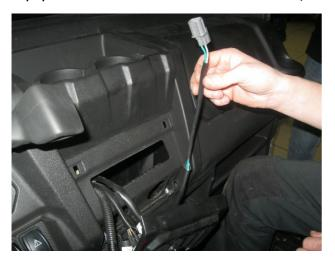
13) Strip the insulation of the white-green shielded wire and connect it with the "controlling" wire of the wiper;
