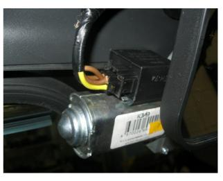
19) Connect the washer fluid tube to the windscreen wiper motor;
