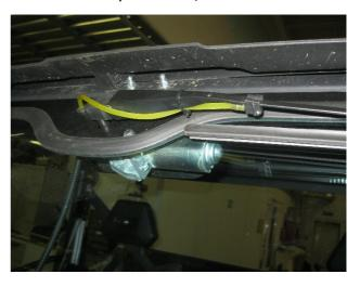
20) Connect the power wires of windscreen wiper to the power clamps on the winch relay;
