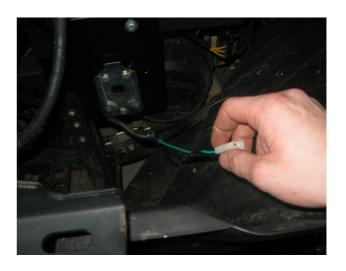
9) Put and screw the ground wire under the bolt of water tank hanger (point 7);
